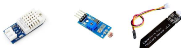
Figure 1. DHT22, LDR, and capacitive moisture probe, left to right.
